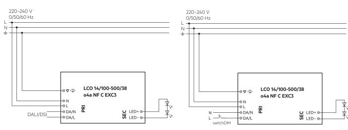
switchDIM with connected LED module
